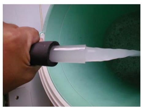
... pour onto the evaporator cavity three liters of fresh water to rinse the molds and the platen.
