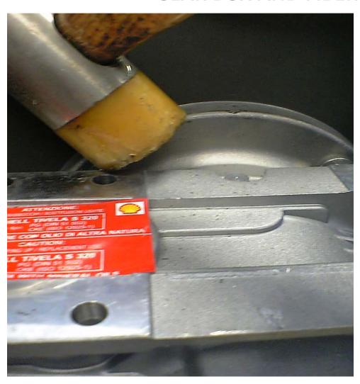
With a mallet, hit a bit the gear box to create some looseness.
