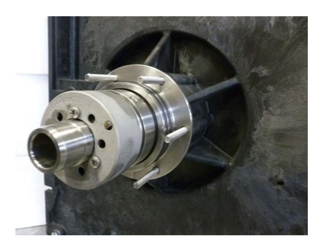
Fit on the drum shaft journal the remaining portion of seal mechanism (stainless steel seal ring with spring), then the space ring .....
