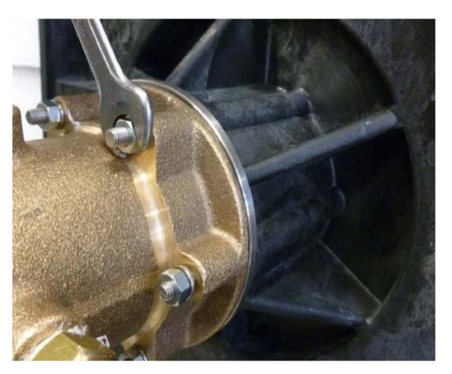
Unloose and remove the 6 nuts and washers securing the refrigerant manifold to the seal mechanism housing.
