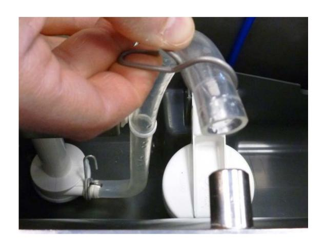
5. Push in water inlet hose clamp and pull the same out from spray system
