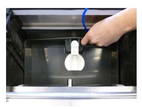
8. Carefully bend and pull the plastic reservoir out from evaporator sink
