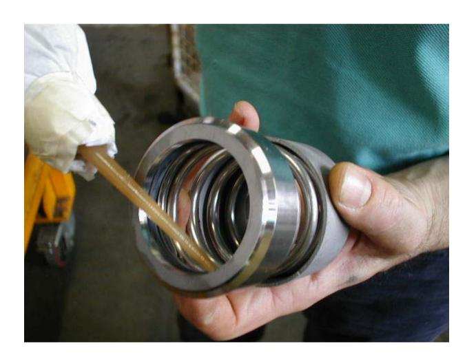
the O ring inner surface of seal mechanism with refrigerant oil.
