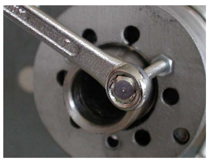
Fit the screw of 4 MA with its nut in one of the three threaded holes then.....
