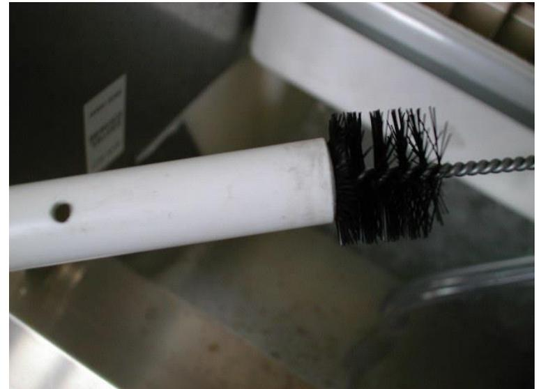
Once properly cleaned re-assembly the Water Distributor Tubes then re-fit it again on the upper side of the evaporator paying attention to match the plastic pin with the hole.
