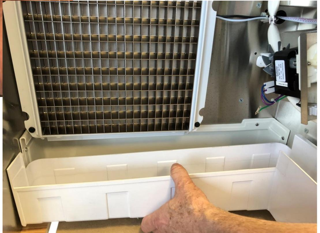
Prepare the cleaning solution by diluting in a plastic bucket two liters of lukewarm water (max 40°C) with 200 ml of **SCOTSMAN Ice Machine Cleaner**.
