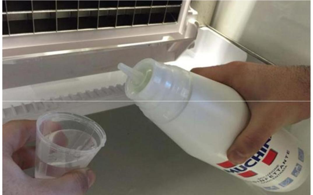
Meanwhile the unit is running the rinsing cycle , mix in a clean bucket some fresh water with 1% of sanitizer product (Amuchina)
