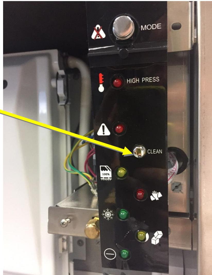
The machine enters in the Cleaning/Sanitize cycle with the red CLEAN LED light on MONITOR PANEL blinking fast in whole procedure
