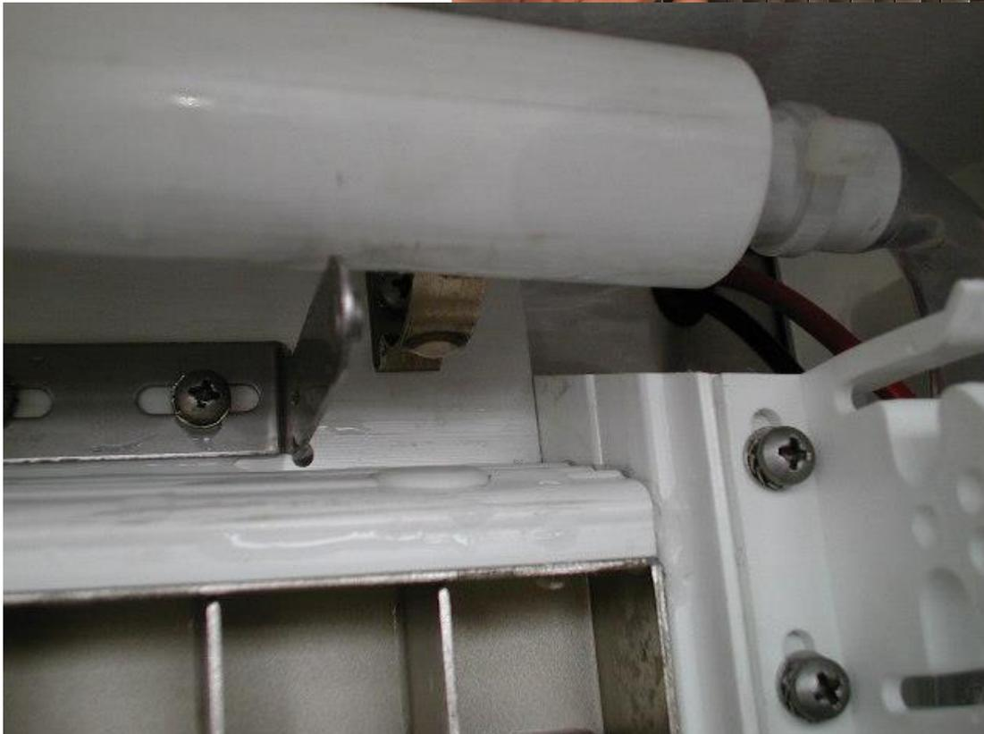
Open up the water distribution tube for cleaning
