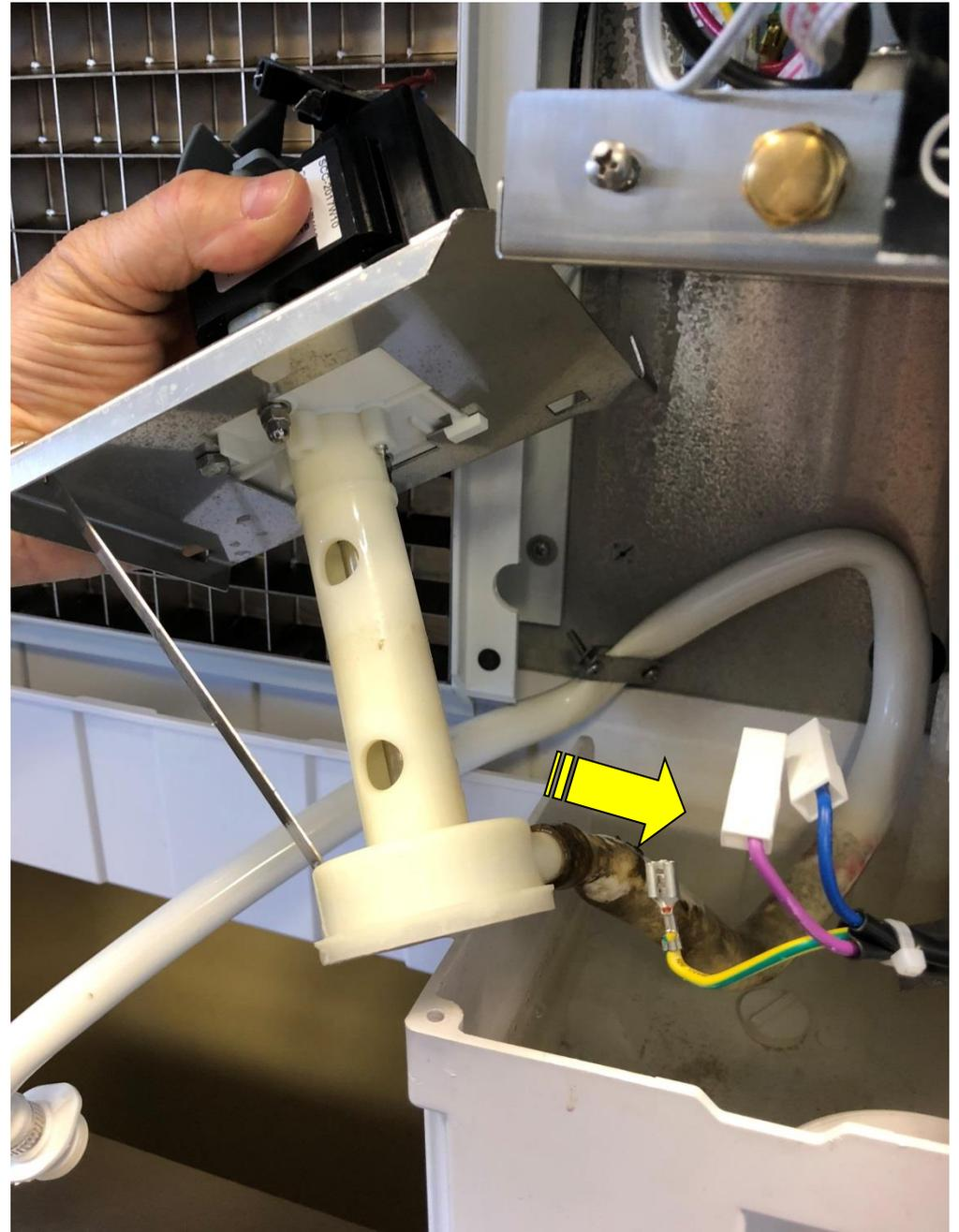
Unscrew the two thumb screws then withdraw reservoir from its seat
