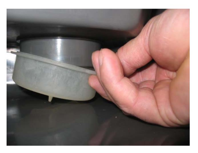
....and remove the soft plastic plug by pulling it down so to drain out all water from the water sump.
