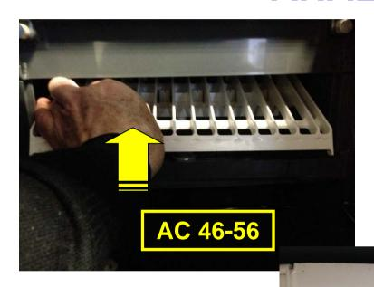
then remove the complete spray platen from the sump and ....
