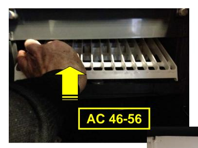
Grasp the spray platen assy on the center spray jet and lift it up so to have access to the water sump.
