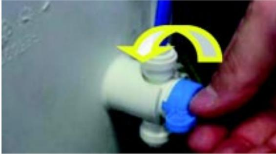
5. Bend down the plastic hose and drain out the water from the water sump than move it up again.
