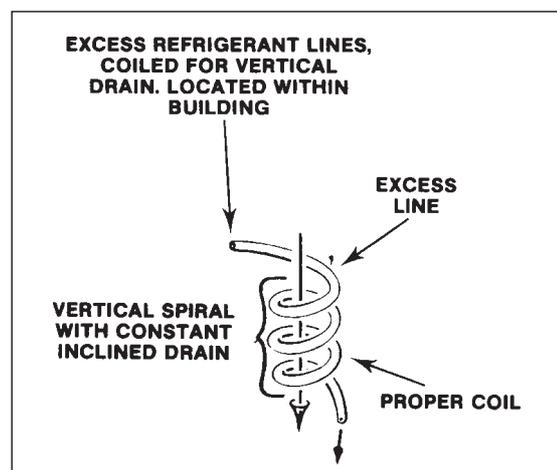
**CAUTION - DO NOT kink or crimp the refrigerant lines. DO NOT bend excess refrigerant lines in a vertical loop (s), which allow trapping of refrigerant in LOW sections during OFF time. Bend and shape excess refrigerant lines in VERTICAL spirals, not HORIZONTAL spirals. See Figure above.**
