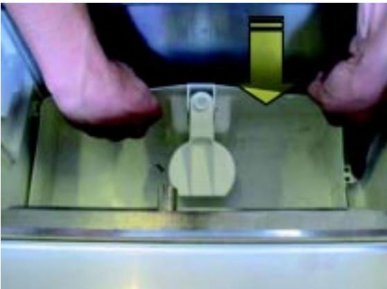
17. Reinstall water pump removed at #6.
