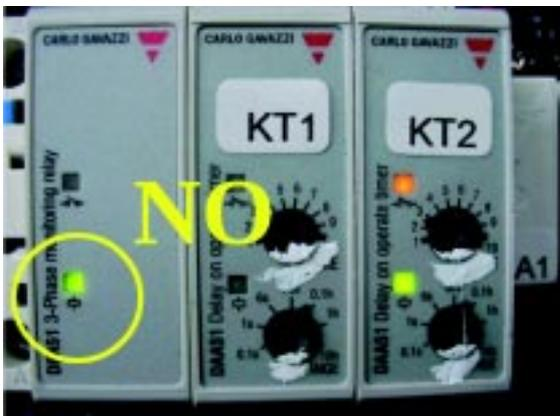
5. Correct wiring is shown by both LEDs Green and Orange steady ON together.
