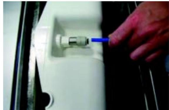
.....and remove water sump from evaporator basin
