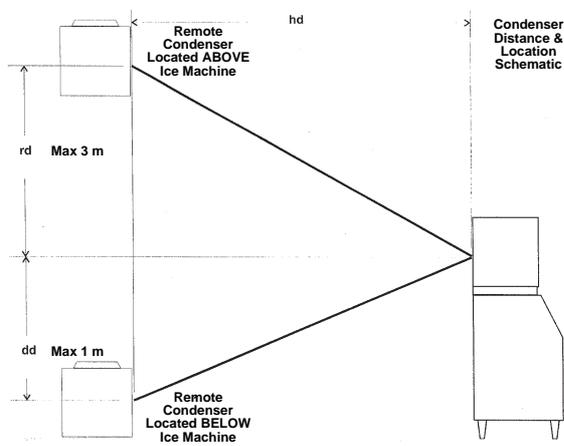
**Location Limits - condenser location must not exceed ANY of the following limits:**
