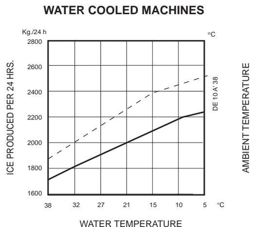
**NOTE.** Daily ice capacity is directly related to condenser air water inlet temperature, water temperature to make ice - and age of machine.
