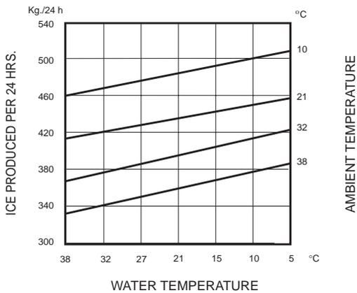
**NOTE.** Daily ice capacity is directly related to condenser air water inlet temperature, water temperature to make ice - and age of machine.
