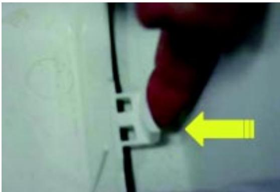
10. By the help of flat screwdriver easily open little bit float valve holding arms and remove it from holders
